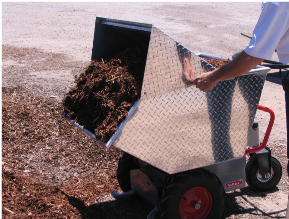
Figure 5. Scoop attachment pivots to permit easy and complete unloading. Scoop is locked in the open position with a ball detent pin.
